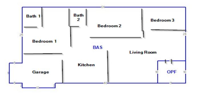
Description of Work: Remove and replace Drywall 4ft high throughout structure Remove and replace all Electrical below 4 ft Remove and replace cabinets in kitchen and bathrooms Remove and replace all (6) interior doors and base Remove and replace carpet and wood flooring through structure Remove and replace plumbing fixtures in kitchen and bathrooms Remove and replace duct work
